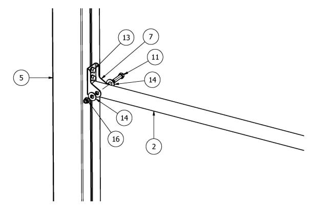
The bottom side of the backstay pipe should be 24" above the bottom of the Side Rail.
