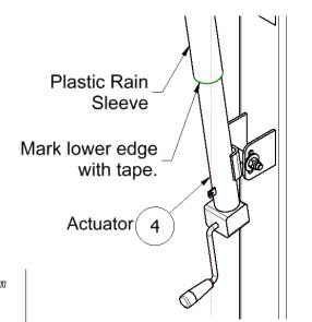
2. Crank the Goal to the minimum height so that the Lifting Arm rests on the stop. Crank clockwise to lower.
