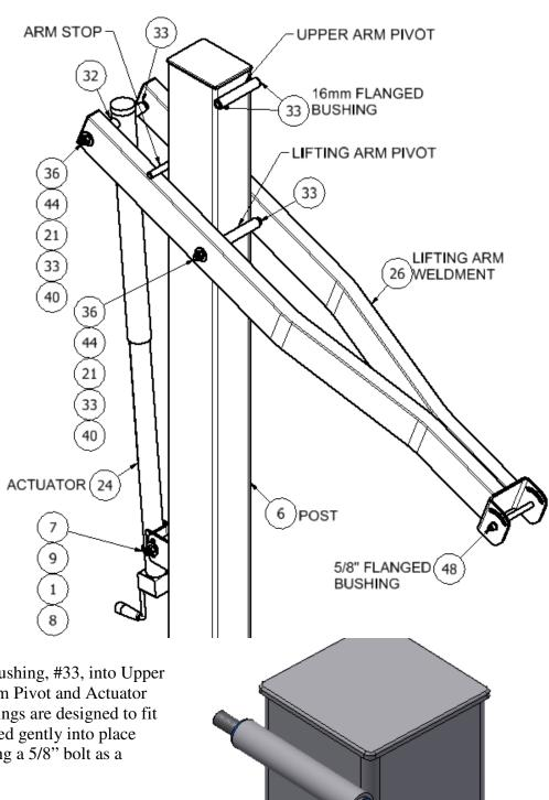
1. Install 16mm Flanged Bushing, #33, into Upper Arm Pivot & Lifting Arm Pivot and Actuator Pivot Tubes, #32. Bushings are designed to fit tightly and must be tapped gently into place with a rubber mallet using a 5/8" bolt as a guide.
