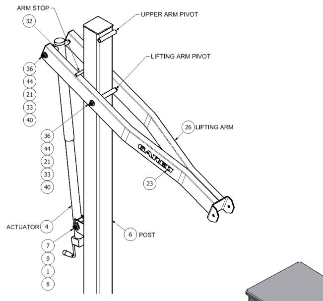
Install 16mm Flanged Bushing, #33, into Upper Arm Pivot & Lifting Arm Pivot and Actuator Pivot Tubes, #32. Bushings are designed to fit tightly and must be tapped gently into place with a rubber mallet using a 5/8" bolt as a guide.
