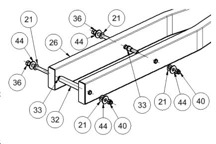
4. Crank the Actuator clockwise to lengthen it until the crank end can be attached to the Anchor on the Post using a 5/8 x 5 1/2" Bolt, #7, and hardware as indicated. Tighten Lock Nut to remove clearance only. **Do not torque**.
