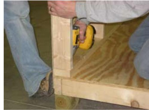
Apply Pressure on outside and secure with 2 1/2" screws.
