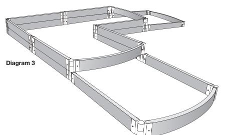
3) Add the second level of the Planter and insert one Stake through the brackets into the aperture on the top of the stake beneath it to lock the second level in place (Diagram 3).
