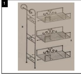
**step1** Attach each tier (A) to left supporting panel (B),using nuts and spanner provided.
