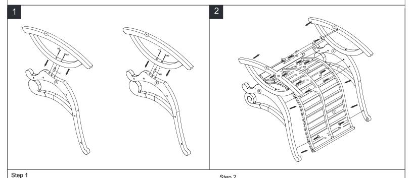
Attached (A) into (B) and using (H1) to put on the hole (H2) tinghten (H4)
