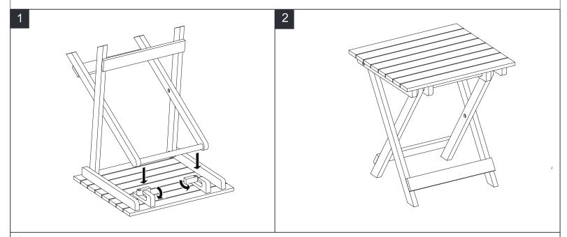
Put leg dow to block and rotate the lock to right side
