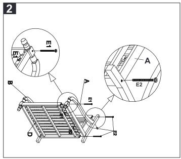
Step 2: put the left side (A) to the chair by using the Allen bolts (E1) and (E2) as shown on the picture. Tighten all with the Alen key (E4).
