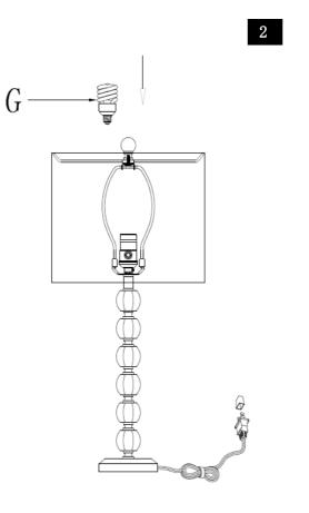
Step2 Insert the bulb(G) into the socket(C).
