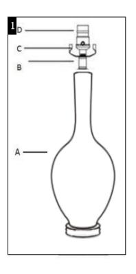
Screw the Neck (B) onto the Lamp base (A)
